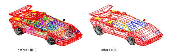
Hiding background lines makes the display much clearer, but you cannot modify hidden-line or render views. It may take a long time to calculate and obscure hidden lines if the drawing is complex. However, you can speed up the process in the several ways. For example, you can avoid drawing details that will not be visible at the scale at which you are displaying or plotting the drawing. You can also exclude objects from the hiding process by zooming into a part of the drawing.
