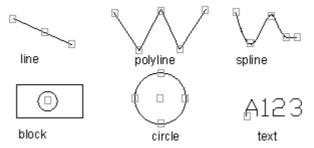
When you perform quadrant grips on circles, the distance is measured from the center point, but not the selected grip. For example, in Stretch mode, you can select a quadrant grip to stretch a circle, and then specify a distance at the prompt of "New circle radius". The distance is measured from the center point, but not the selected quadrant. If you select the center point, the circle moves.
