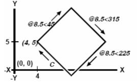
Drawing a tilted square using the relative polar coordinates method; enter *C* to close.
