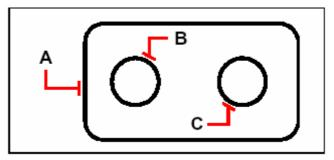
To calculate the area of the gasket using the Area command, first add the area of the entire gasket (**A**), and then subtract the areas of the two circles (**B** and **C**). As you select objects, the program displays the calculations. If the command bar is displayed, the information appears there. If the command bar is not displayed, the program opens the Prompt History window and displays the calculations.
