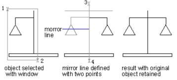
System variable MIRRTEXT affects texts created with MIRROR command. When MIRRTEXT is on, the text object is processed the same as the other objects. When MIRRTEXT is off, the direction of text objects keeps unchanged. Displaying as follows:
