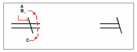
Select the boundary edge (**A**), and then specify the first Result. point (**B**) and second point (**C**) of the fence.
