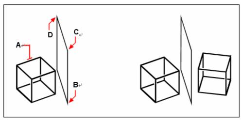
Select the object to mirror (**A**), and then specify The resulting mirrored object. the first point (**B**), second point (**C**), and third point (**D**) defining the mirror plane.
