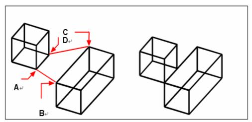
Select the objects to align, and then specify the first source point (A), the first destination point (B) the second destination point (C) and the sec
