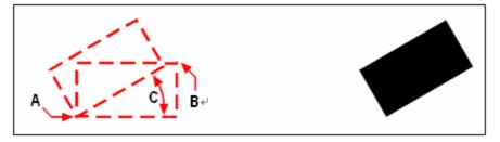
Opposite corners (A and B) and rotation angle (C). Resulting plane.
