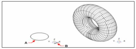
Select the object to revolve (**A**) and the axis (**B**) about The resulting revolved solid. which to revolve it. followed by the angle of revolution.
