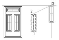
In addition to specifying base point or displacement point on the drawing, you can also type coordinate value on the command line. The Vector option is also used to define a new position.
