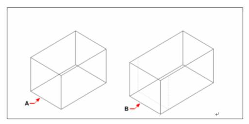
Select the entity to extrude, and then specify the face(s) to extrude (**A**), and the height of extrusion or path. The resulting entity with the face extruded to position (**B**).
