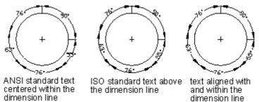
The justification and other settings may affect the vertical alignment of text. If you select Horizontal Alignment, text inside the extension lines and centered within the dimension is placed horizontally, as shown in the leftmost figure above.
