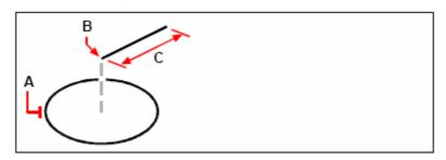
You can use point filters to draw a line by first selecting a point in the xy plane (**A**), specifying the z coordinate (**B**), and then specifying the length of the line (**C**).
