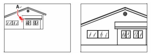
Current view(left) showing the point to be centered in the new view (A), and the new view(right) zoomed using a scale factor of 2x
