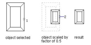
You can also scale objects by comparing the basic scale and new scale. The objects become larger if the new scale is large than the basic scale.
