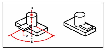
Select the objects to rotate (**A**), specify the endpoints of the axis of rotation (**B** and **C**), and then specify the rotation angle (**D**).
