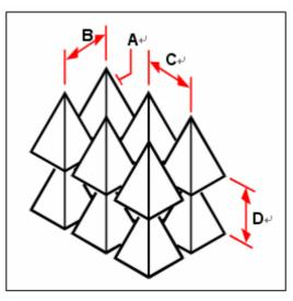
To create a three dimensional rectangular array, select the object to copy (A), type the number of rows, columns, and levels, and then specify the distance between each row (B), column (C),and level (D).
