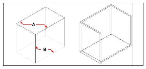
Select the entity, and then select faces to remove (**A**) and (**B**), then specify an offset distance.
