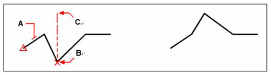
Select the polyline (**A**), move the current vertex marker to the vertex you want to move (**B**), and then specify the new vertex location (**C**).
