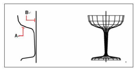
Select the object to be revolved (**A**) and the The resulting revolved surface mesh. axis of revolution (**B**).
