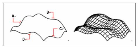
Select the objects to be used as the four The resulting Coons surface patch mesh. edges (**A**, **B**, **C**, and **D**).
