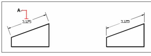
Select the dimension to be made oblique (**A**), and then type the obliquing angle.
