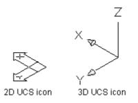
Displaying 2D or 3D UCS icon is controlled by the UCSICON command. You can display the UCS icon at the UCS origin point to indicate the origin and orientation of the current UCS using the UCSICON command.
