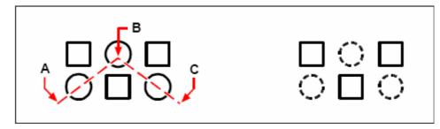
Fence by specifying the endpoints of the fence segments (**A**, **B**, and **C**).
