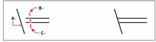
Select the boundary edge (**A**), and then specify the Result. first point (**B**) and second point (**C**) of the fence.
