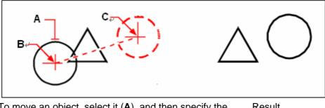
To move an object, select it (**A**), and then specify the Result base point (**B**) and the displacement point (**C**).
