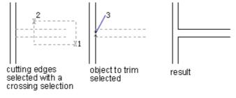
Using variable selection methods while trimming several objects can help you select edges or objects more easily.
