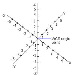
Generally, the WCS and the UCS are coincident with each other, which means that their axes and origin points are overlapped exactly. No matter how many times you relocate the UCS, you can always use the World option of the UCS command to make it coincident with the WCS.
