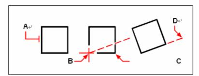
To rotate an entity in reference to a base angle, select the entity (**A**), specify base point (**B**), select the reference angle and pick point (**B**) again (or type the @ symbol), specify the second point (**C**), and then specify the point representing the new angle (**D**).
