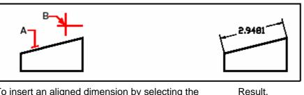
To insert an aligned dimension by selecting the entity, select the entity (**A**) to dimension, and then select the dimension line location (**B**).
