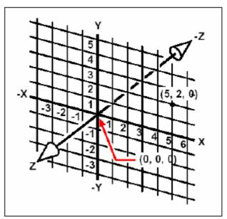
Point 5,2,0 is 5 units to the right (along the x axis), 2 units up (along the y axis), and 0 units (along the z axis) from the origin (the 0,0,0 point) Settings such as snap and entity snap allow you to draw accurately without specifying coordinates.
