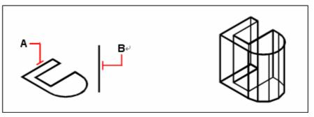
Select the object to extrude (**A**) and the The resulting extruded surface mesh. extrusion Path (**B**).
