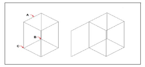
Specify the face(s) to copy (**A**), the base The resulting entity with the face copied. point (**B**), and the end point(**C**).
