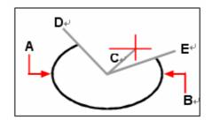
First axis endpoint (**A**), second axis endpoint (**B**), half length of other axis (**C**), start angle of arc (**D**), and end angle (**E**).
