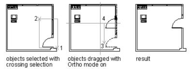
From the picture above, the Door is contained entirely in the selection window, so the door can be moved to the specified location. And the wall lines are only partially within the selection area, as a result, the door moves with the wall.
