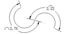
Additionally, orthogonal or radial extension line is available for arc length dimension, only the included angle of the arc segment selected for creating arc length dimension is smaller than 90 degree can display it's orthogonal extension line.
