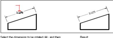
Select the dimension to be rotated (A), and then type the rotation angle.
