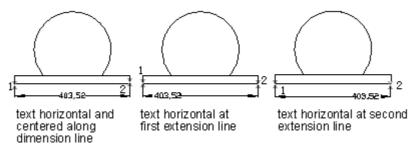
If the "place text manually when dimensioning" option on the Fit tab of the Modify Dimension Style dialog box is chosen, as you create dimensions, you can place the dimension anywhere inside or outside the extension lines along the dimension line. This option is useful when the space between the extension lines is limited.
