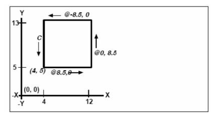
Drawing a square using the relative Cartesian coordinates method; enter *C* to close. The first relative coordinate (@8.5,0) locates the new point 8.5 units to the right (along the x axis) from the previous point of 4,5; the second relative coordinate (@0,8.5) locates the next point 8.5 units above (along the y axis) the previous point, and so on. Entering C (for Close) draws the final line segment back to the first point specified when you started the Line command.
