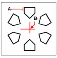
To create a polar array, select the object to copy  $(\mathbf{A})$ , specify the center point of the array  $(\mathbf{B})$ , and then specify the number of items to array, the angle the array is to fill, and whether to rotate the items.
