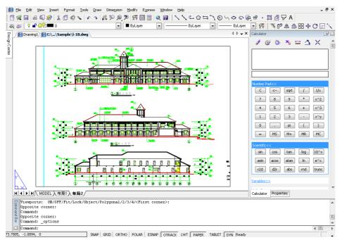
When you're ready to print or plot your drawing, you can switch to paper space on a Layout tab, where you provide a layout of the drawing as you want it to appear on a sheet of paper.
