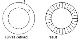
If you select a closed polylines, the ruled surface begins at the last vertex and proceeds backward along the polyline segments. If you select open curves, selecting objects at the same side of the two objects to create ruled surface, selecting objects at different side of the two objects to create crossed ruled surface, shown as follows:
