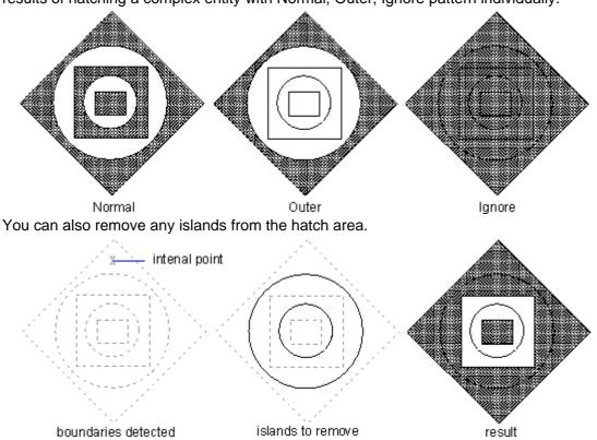
Ignore internal objects, only hatches outer objects. The following example displays the results of hatching a complex entity with Normal, Outer, Ignore pattern individually:
