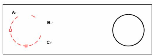
To scale using grips, select the object (**A**), click a grip (**B**), and Result. scale the object by dragging the grip to its new location (**C**).
