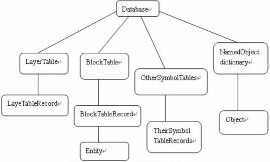
Fig2 Key elements of ZWCAD database
