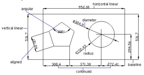
When you create a dimension, the program draws it on the current layer, using the current dimension style. Each dimension has an associated dimension style, which controls the appearance of the dimension, such as the types of arrowheads, text style, and colors of various components. You can modify existing dimension styles by changing one of the dimension variable settings and then updating the dimension style to reflect the new settings.
