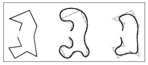
Original polyline After applying Fit curve. After applying Spline.
