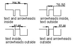
If there is no space for text between the extension lines, the system creates a leader automatically to place text. You can set the relationship between them on the Text tab of the Modify Dimension Style dialog box.
