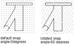
The snap base point is the offset from a specific X, Y value on the current UCS. The default snap base point is 0, 0, but you can change it to any X, Y coordinate value to adjust snap points. Changing snap base point does not affect grids.
