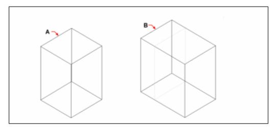
The resulting object with the face offset to position (B).
