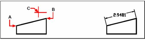
To insert an aligned dimension by selecting the extension line origins, select the first extension origin (**A**), select the second extension origin (**B**), and then specify the dimension line location (**C**).
