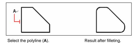
Before creating fillets, you should ensure the distance between each vertex is long enough to accommodate the fillet radius in order to insert a fillet arc.
