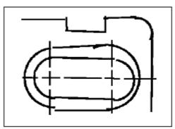
Paper based drawings lack the high degree of accuracy possible when using CAD. Lines often overlap or fail to meet adjacent lines.
