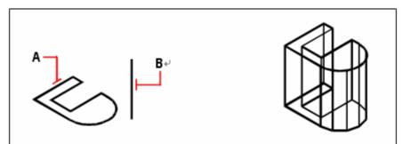
Select the object to extrude (**A**) and The resulting extruded surface mesh. the extrusion path (**B**).
