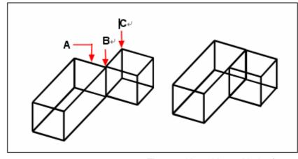
Specify the face(s) to move(A), the The resulting object with the face base point (B),and the end point moved to the new position.(C)
