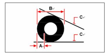
Width (A) and diameter (B) of the donut and tangent objects (C).
