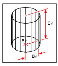
Center of the base (A), radius of the base (B), and the height (C).
