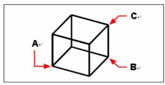
First corner of the base (A), the opposite corner of the base (B), and the height (C).
