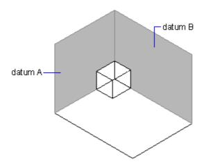
In the illustration above, the axis formed by the point where datums A and B intersect called the datum axis. The position of the pattern is calculated from that axis.
