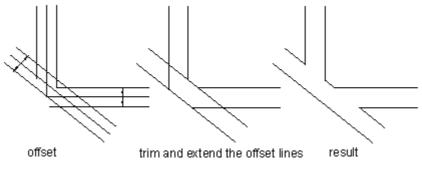
If the objects to offset are 2D polyline or spline, the system trims them automatically when the specified distance is larger than can otherwise be accommodated. Displaying as follows:
