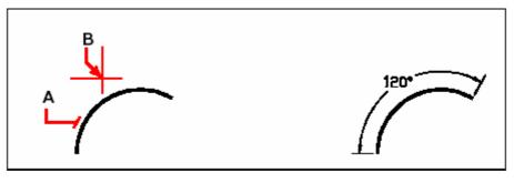
To dimension the angle subtended by an arc, Select the arc (**A**), and then specify the dimension arc location (**B**). Result.
