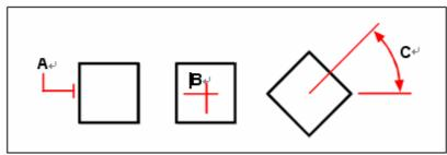
To rotate an object, select the object to rotate (A), and then specify base point (B) and the rotation angle (C).
