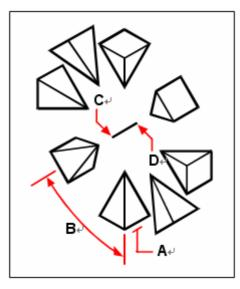
To create a three dimensional polar array, select the object to copy (**A**), type the number of items to array, specify the angle the array is to fill (**B**), and then specify the center point of the array (**C**) and a second point along the central axis of the array (**D**).
