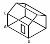
Define the new UCS by selecting the origin (**A**), a point on the positive x-axis (**B**), and a point in the positive y direction (**C**).
