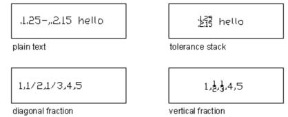
You can also use Stack button on the Text Formating toolbar to create stacked text.
