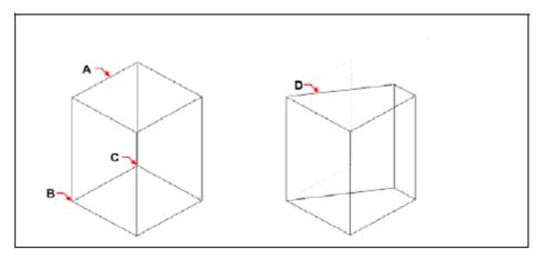
Specify the face(s) to taper (**A**), a base point(**B**), a second point along the taper axis(**C**), and a taper angle.
