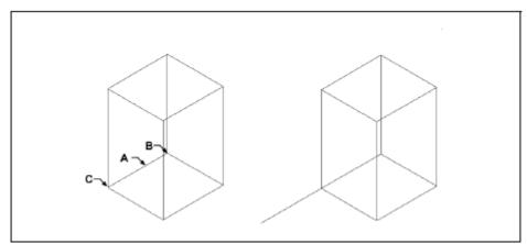
Specify the edge(s) to copy (**A**), the base point (**B**), and the end point(**C**).
