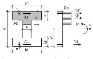
$\sigma_{s}$  and  $\sigma_{s}'$  are stresses in bottom and  $\mathbf{R}_{sc} \leq \sigma_{si} = -\frac{1 - \omega \mathbf{y}_{si} / \mathbf{x}}{1 - \omega / 1.1} \cdot \sigma_{sc,u} \leq \mathbf{R}_{sc} \quad \begin{vmatrix} \mathbf{y}_{si} = \mathbf{h}_{0} - 3a \sigma_{s} \\ \mathbf{y}_{si} = \mathbf{a}' - 3a \sigma_{s}' \end{vmatrix}$
