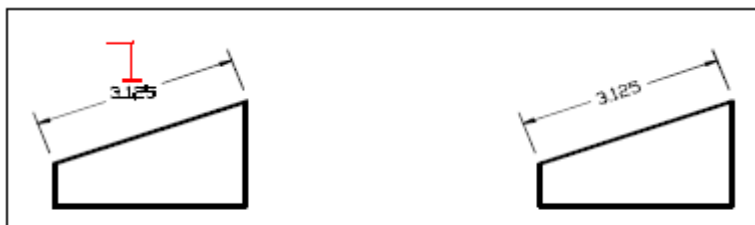
Select the dimension to be rotated (A), and then type the rotation angle.
