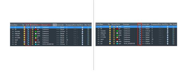
Figure 23. Changing column order in the Layer Properties Manager by dragging
